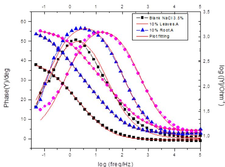
**Fig. 5.** Bode plots for mild steel in 3.5% NaCl medium without and with 10% of leaves extract and root extract from *Anabasis Aretioïdes* plant
