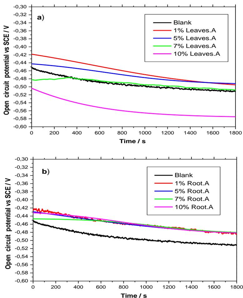
**Fig. 2.** Variation of the open-circuit potential (OCP) of the mild steel substrate in a neutral solution at various concentration of a) leaves methanolic extract and b) root methanolic extract from *Anabasis Aretioïdes* plant
