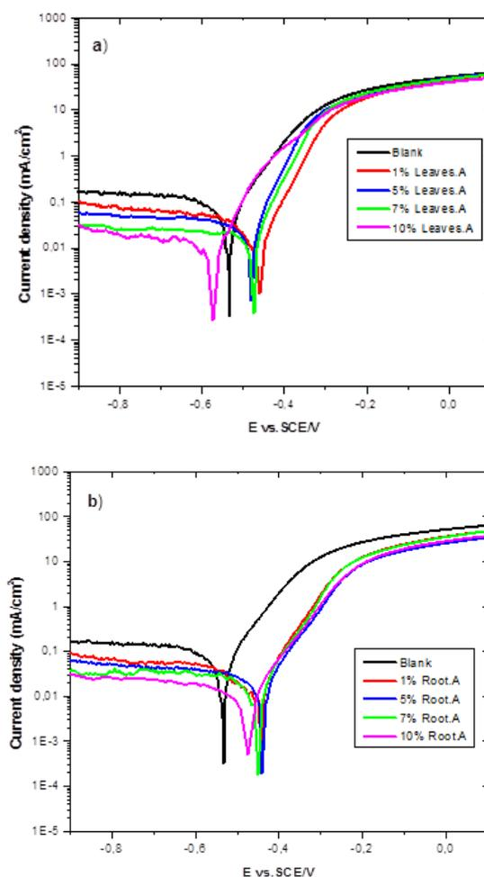
**Fig. 3.** Potentiodynamic polarization curves for mild steel in 3.5% NaCl solution without and with different concentrations of a) leaves and b) root methanolic extracts from *Anabasis Aretioïdes* plant
