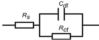
**Fig. 6.** the equivalent circuit model used to fit EIS experiment data
