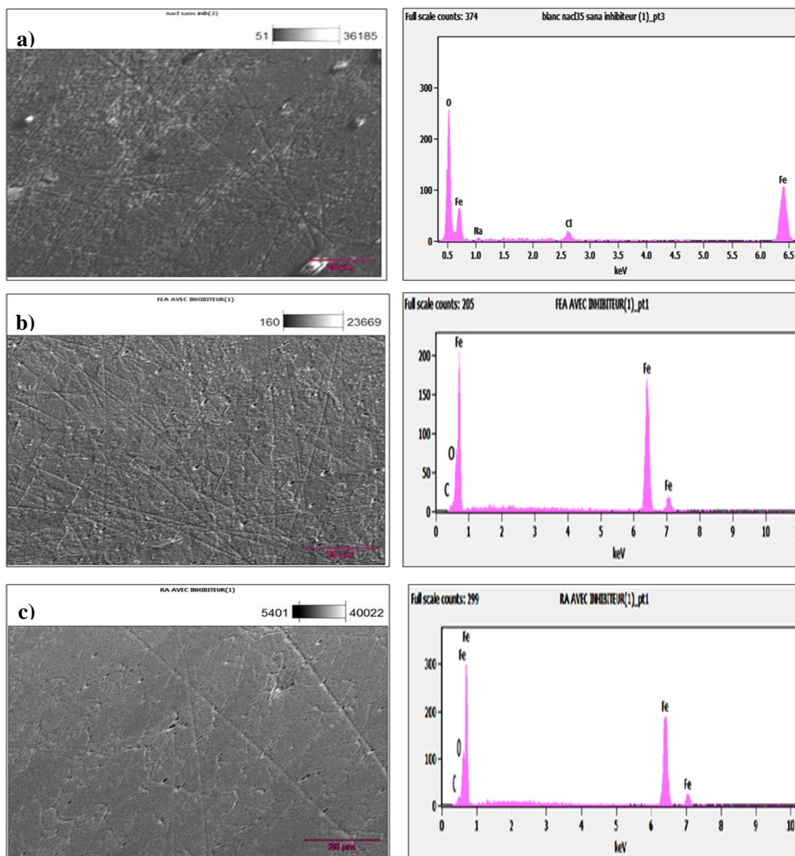
**Fig. 7.** SEM photograph and Spectrum of EDS analysis of E24 steel immersed for 24 hours, in NaCl 3.5% without (a) and with 10% of methanolic extracts of leaves (b) and root (c) parts from *Anabasis Aretioïdes* plant
