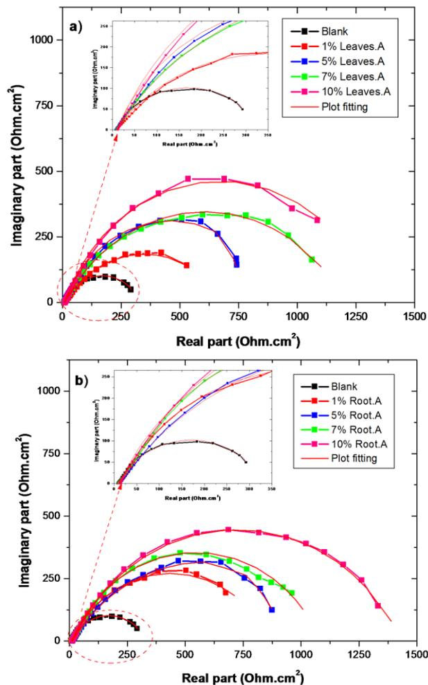
**Fig. 4.** Nyquist plots recorded for mild steel substrate in 3.5% NaCl medium in the absence and the presence of various concentrations of a) leaves methanolic extract and b) root methanolic extract, parts from *Anabasis Aretioïdes* plant
