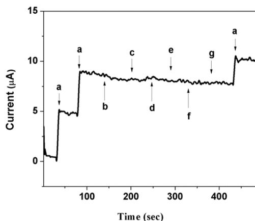
**Fig. 12.** Amperometric *i-t* response for the addition of a) 0.05 uric acid and 0.1  $\mu\text{M}$  of (b) glucose, (c) ascorbic acid, (d)  $\text{H}_2\text{O}_2$ , (e) Glycine, (f) Tyrosine, and (g) L-Cysteine, in pH 7 PBS at GCE/ DBCMAT-CoPc (applied potential of 0.5 V)
