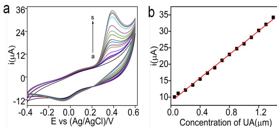
**Fig. 8.** CVs plot of; (a) modified GCE of Different concentrations (0.1-1.8  $\mu\text{M}$ ) of uric acid, at scan rates 50 mV/s and (b) Linear plot of peak current vs concentration of uric acid
