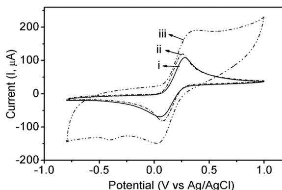
**Fig. 7.** Charge transfer behavior of the **i)** bare GCE and **ii)** GCE/DBCMAT-CoPc and **iii)** GCE/DBCMAT-CoPc-MWCNT electrodes in phosphate buffer with 0.1 mM  $\text{K}_4[\text{Fe}(\text{CN})_6]$  at  $50 \text{ mV s}^{-1}$
