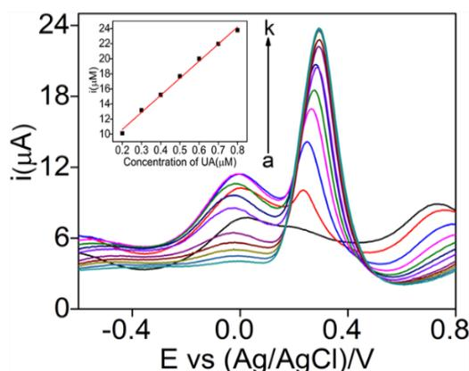
**Fig. 10.** Experimental DPV peaks at modified electrode and Different concentrations of uric acid and inset linear plot of positive peak current vs different concentrations of uric acid/ $\mu\text{M}$
