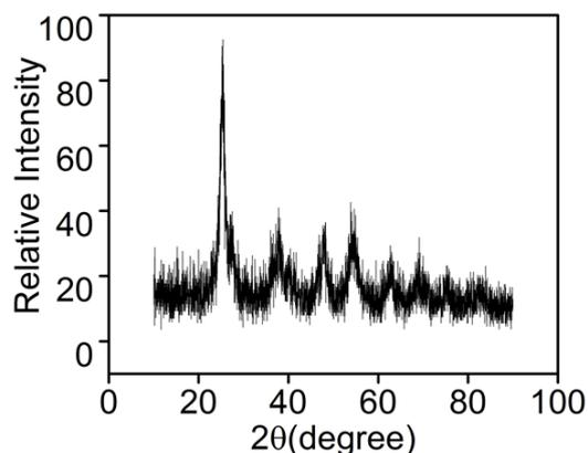
**Fig. 5.** X-ray diffractograms of DBCMAT-CoPc
