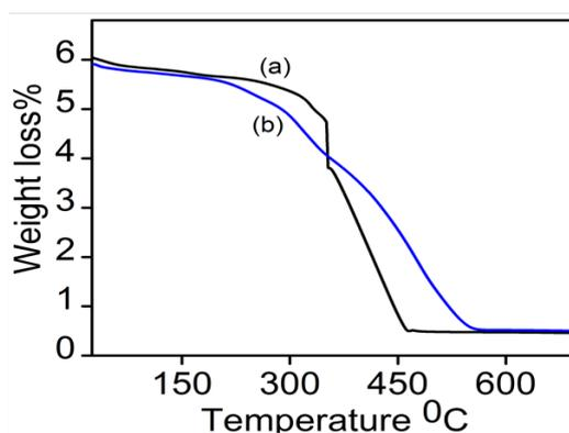
Fig. 4. TGA of (a) CoTcPc (b) DBCMAT-CoPc
