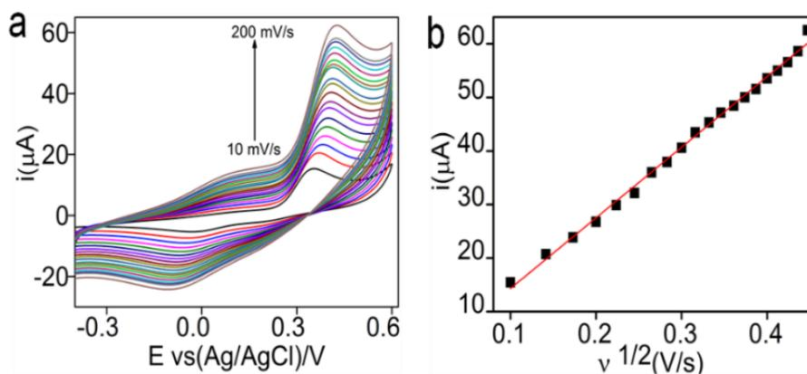
**Fig. 9.** Experimental CVs peaks at: (a) Different scan rates of uric acid (10-200  $\text{mVs}^{-1}$ ) and (b) Linear plot of peak current v/s different scan rates/ $\text{mVs}^{-1}$
