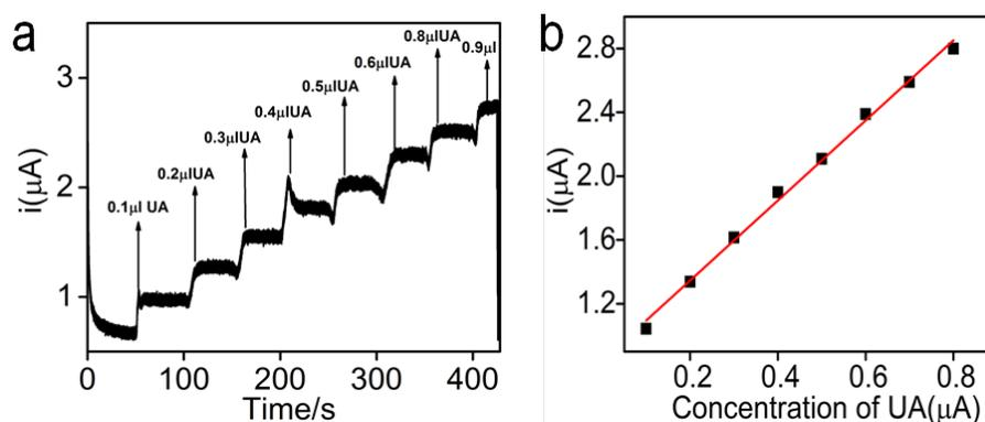
**Fig. 11.** An experimental Amperometry uric acid peaks at: (a) Different concentrations of uric acid and (b) Linear plot of  $I_p$  v/s different concentrations of uric acid. Applied potential +0.5V
