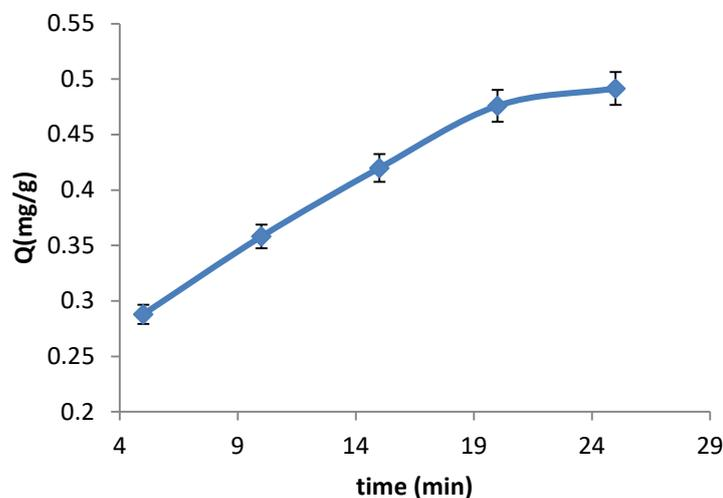
Fig. 5. Optimization of adsorption time for nano-MIP
