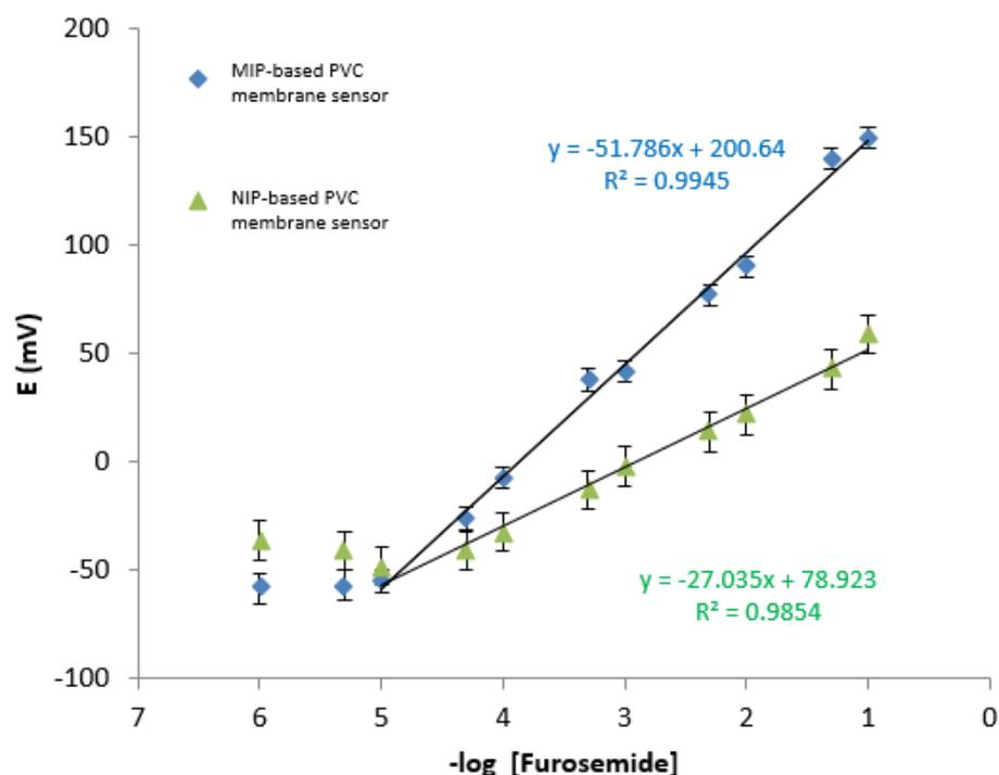
**Fig. 6.** Calibration curve of the potentiometric sensor based on nano-MIP and NIP
