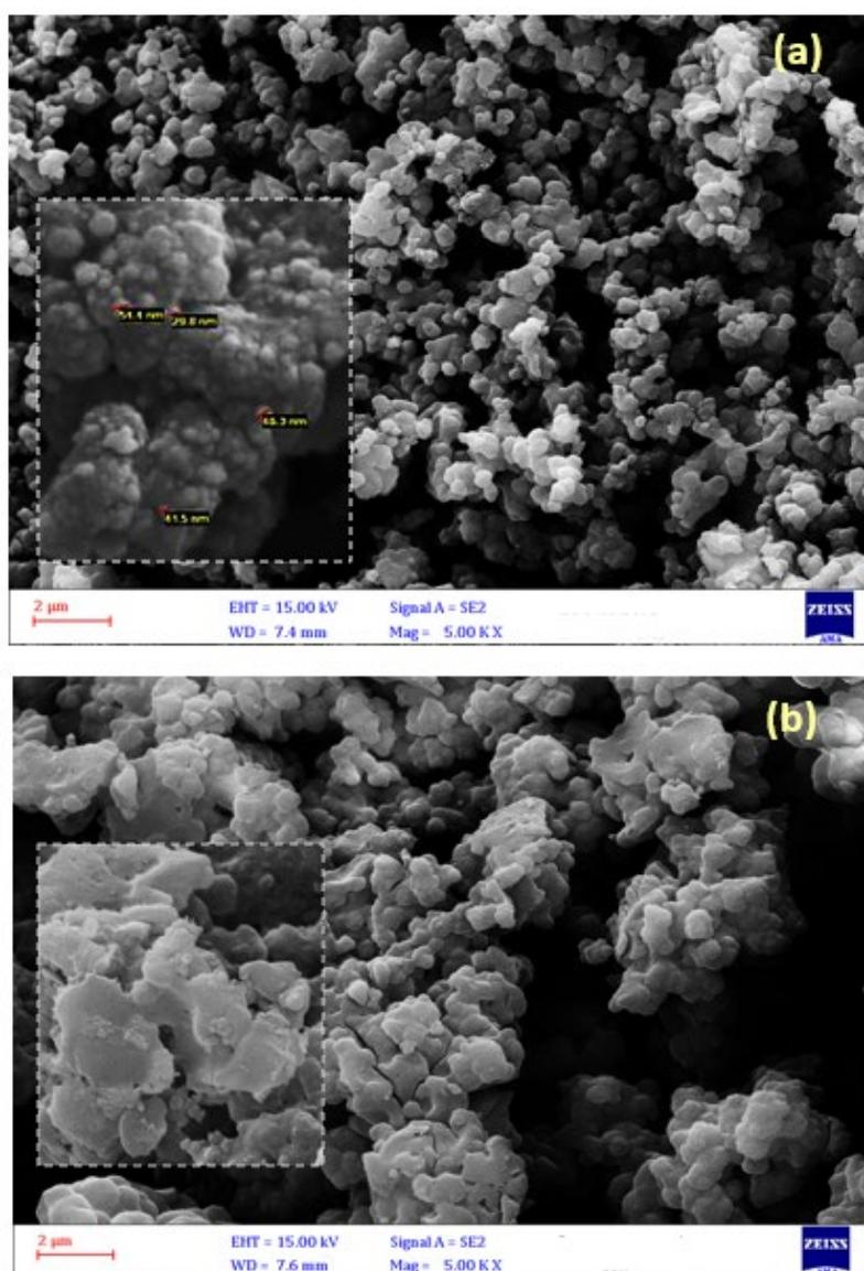
Fig. 2. SEM images of (a) prepared nano-MIP and (b) NIP
