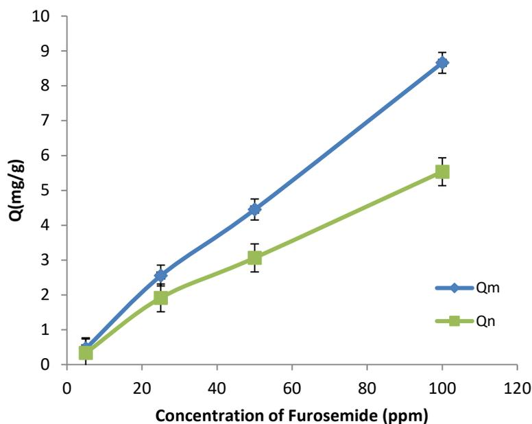
**Fig. 4.** Static adsorption of nano-MIP and NIP for Furosemide
