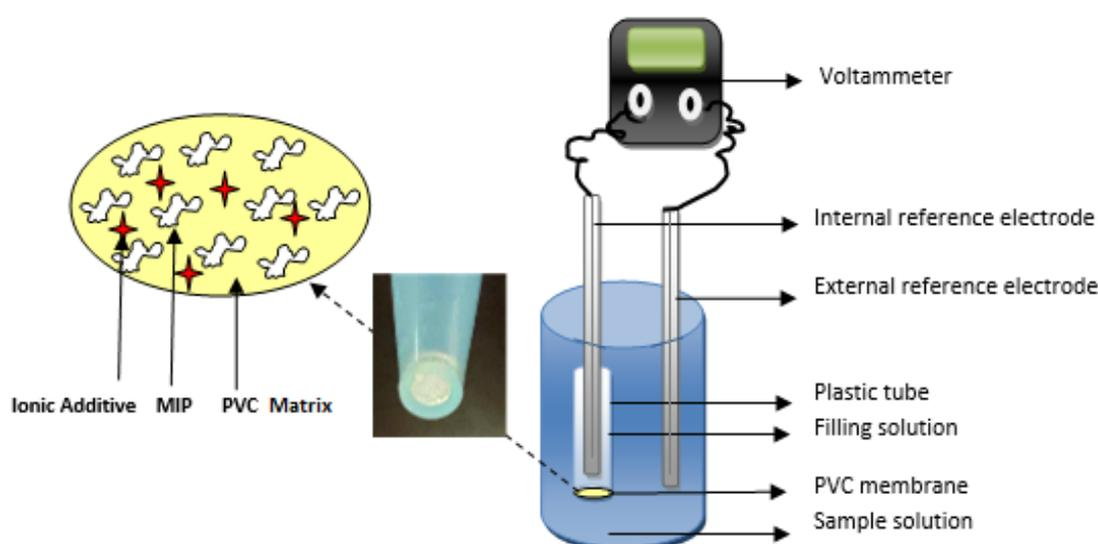
**Scheme 1.** Schematic of electrode preparation
