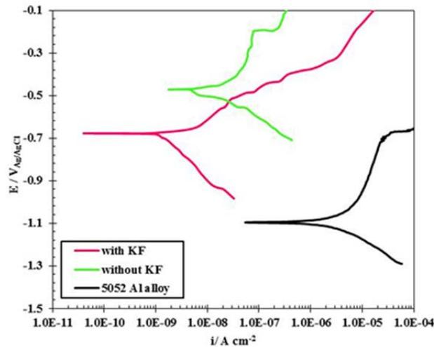
**Fig. 4.** Potentiodynamic polarization curves of 5052 aluminum alloy samples with PEO coatings for A, A' and base samples in the test (3.5% NaCl) solution.
