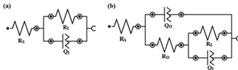
**Fig. 6.** Electrical equivalent circuit for the simulation of 5052 aluminum alloy with PEO coatings for A, A' and base samples
