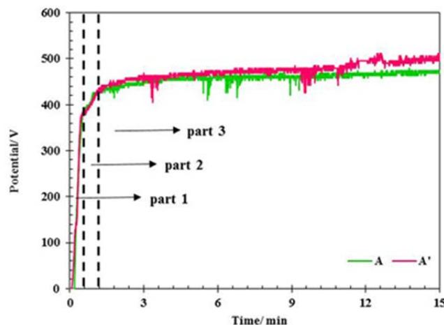
**Fig. 1.** Voltage-time plots of 5052 aluminum alloy samples during PEO coatings in electrolytes with and without KF addition under DC condition for 15 min applying a frequency of 50 Hz
