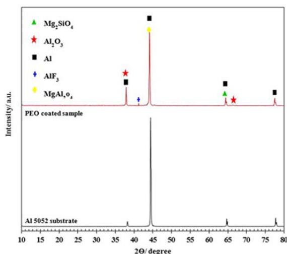
**Fig. 3.** XRD patterns of the 5052 aluminum alloy and PEO-coated sample in  $12 \text{ g.l}^{-1}$  sodium silicate concentration,  $2 \text{ g.l}^{-1}$  KOH with  $2 \text{ g.l}^{-1}$  KF
