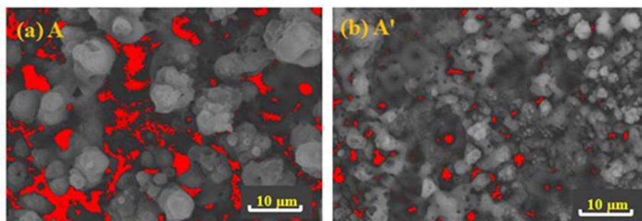
**Fig. 7.** The percentage of porosity in A and A' samples
