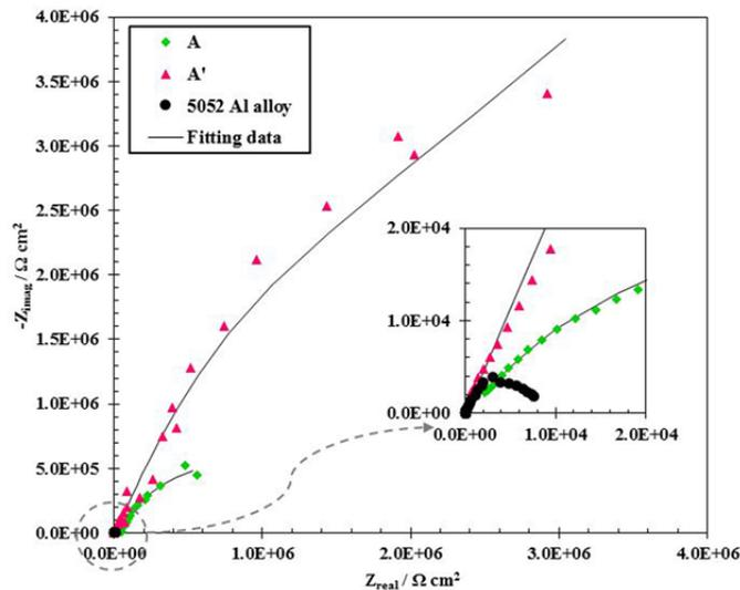
**Fig. 5.** Nyquist plots of 5052 aluminum alloy samples with PEO coatings for A, A' and base samples in the test solution.
