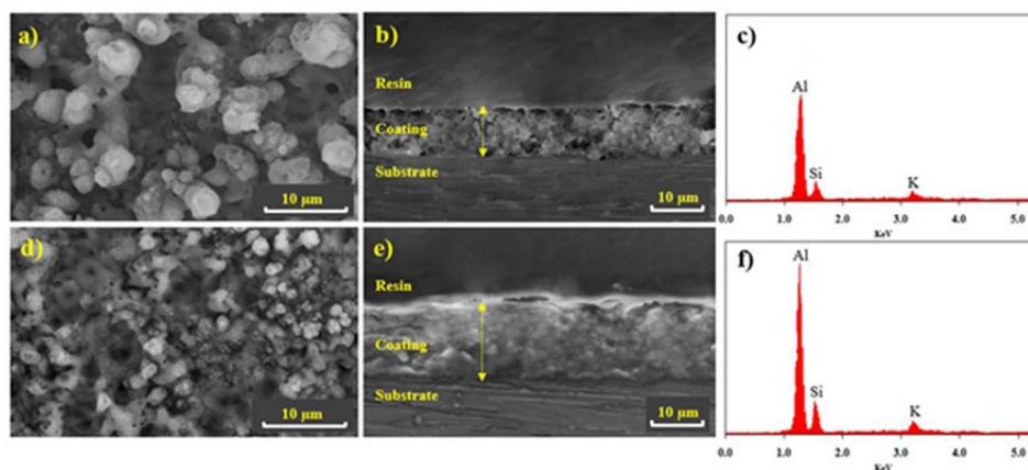
**Fig. 2.** Surface morphologies (a, d), cross-section images (b, e) and EDS of the oxide layer (c, f) of 5052 aluminum alloy samples with PEO coatings in presence and absence of KF in electrolytes (A, A') respectively
