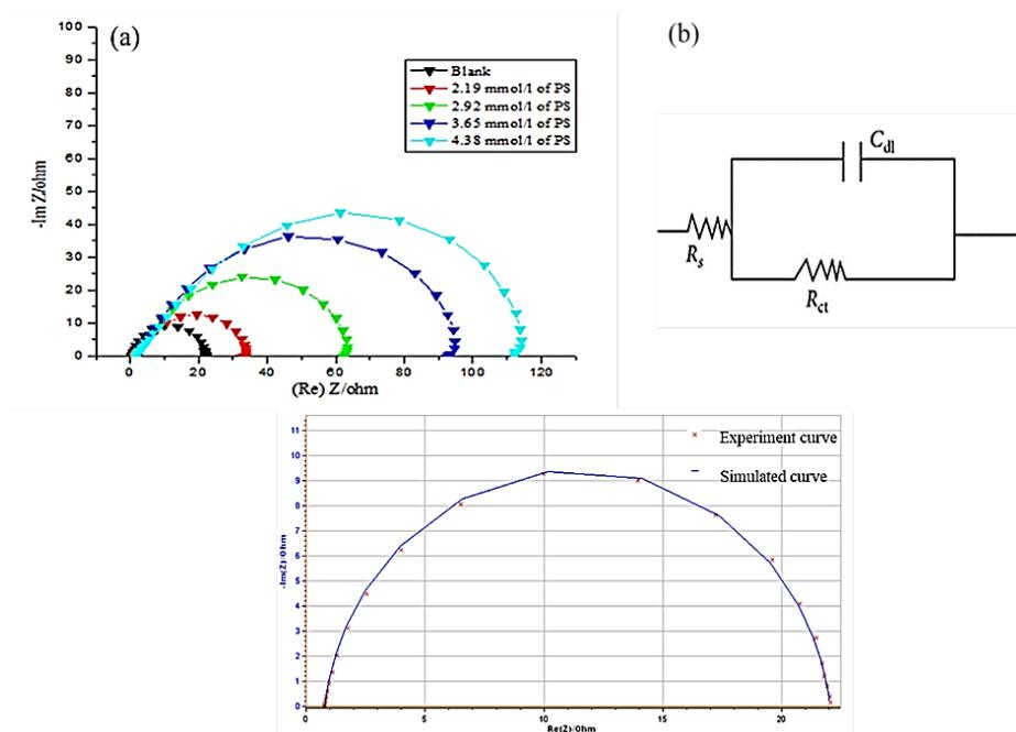
**Fig. 4.** (a) Nyquist plots of E24 steel in 1 M HCl with different concentrations of PS coating; (b) Electrical circuit equivalent to the metal/PS/HCl interface and (c) Nyquist plot fitted using the electrical circuit
