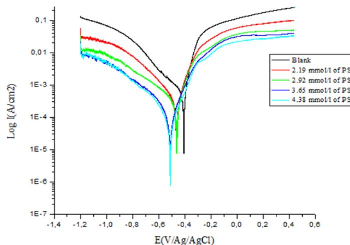
**Fig. 2.** Polarization curves of carbon steel in 1 M HCl in the absence and the presence of different concentrations of PS coating at 298 K
