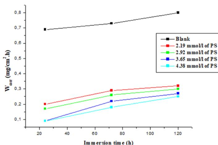
Fig. 2. Variation of corrosion rate with immersion time for different polystyrene concentration
