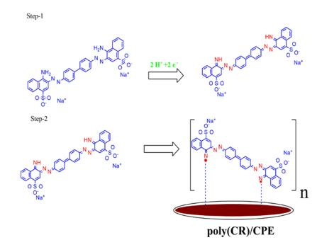
Scheme 1. Mechanism for electrolytic oxidation of TR at the (poly congo red) MCPE
