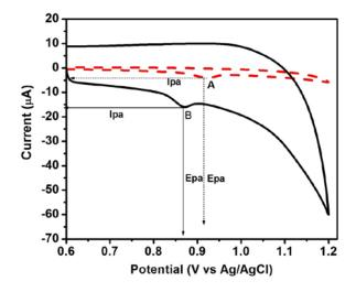
**Fig. 4.** Cyclic voltammograms obtained for the oxidation of 0.025 mM TR in 0.1 M PBS (pH 7.0) at BCPE (dotted line) and Poly CR/CPE (thick line) Scan rate: 50 mV/s
