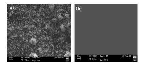
Fig. 2. SEM images of (a) BCPE; (b) Poly CR/ CPE
