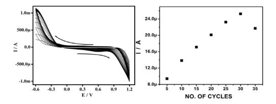
**Fig. 3.** (a) Cyclic voltammograms for the electrochemical polymerization of 1 mM Congo Red on a carbon paste electrode at the scan rate of 50 mVs<sup>-1</sup>; (b) Dependence of the oxidation peak current of 0.025 mM TR on the number of voltammetric scans
