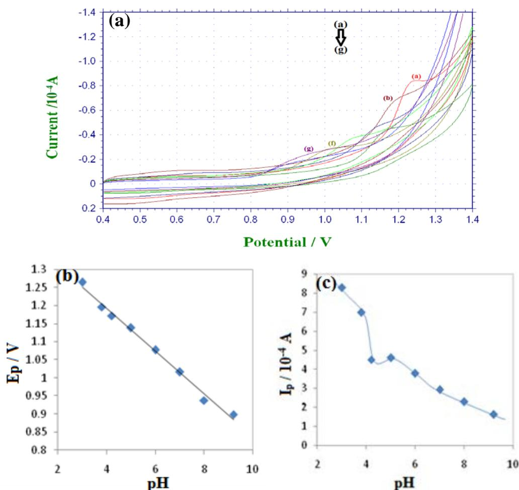
**Fig. 3. a)** Effect of pH on the peaks in phosphate buffer solution at (a) pH 3.0, (b) pH 4.2, (c) pH 5.0, (d) pH 6.0, (e) pH 7.0, (f) pH 8.0 and (g) pH 9.2 with potential scan rate 50 mVs<sup>-1</sup>. Other conditions are as in Fig. 1; **b)** Effect of pH on the peak potential of TP; **c)** Effect of pH on the peak current of TP
