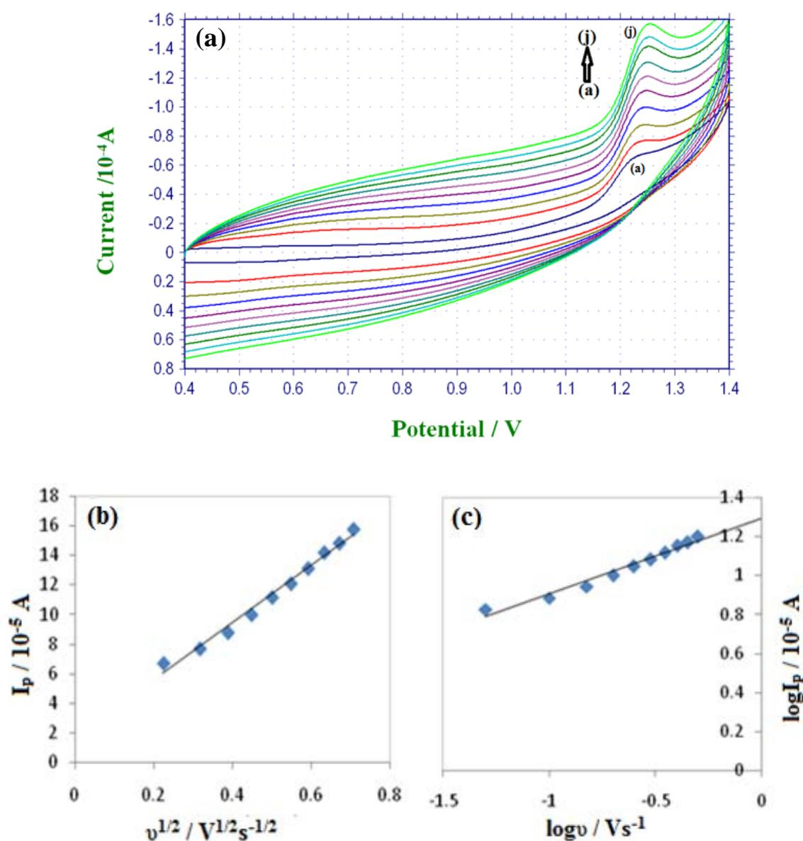
**Fig. 4.** a) Cyclic voltammograms obtained for 1.0 mM TP in PBS of pH 3 at scan rates of (a) 0.05, (b) 0.1, (c) 0.15, (d) 0.2, (e) 0.25, (f) 0.3, (g) 0.35, (h) 0.4, (i) 0.45 and (j) 0.5 Vs<sup>-1</sup>; b) Dependence of the oxidation peak current on the square root of scan rate; c) Dependence of the logarithm of peak current on logarithm of scan rate
