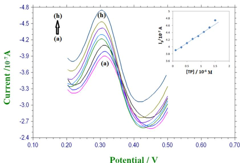
**Fig. 5.** Differential pulse voltammograms of GPE/CTAB in TP solution at different concentrations of (a) 0.1, (b) 0.3, (c) 0.5, (d) 0.7, (e) 9.0, (f) 1.1 (g) 1.3 and (h) 1.5  $\mu\text{M}$
