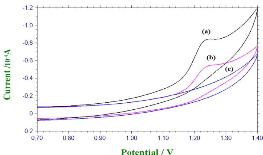
**Fig. 1.** Cyclic voltammograms with pH 3, 0.2 M PBS,  $v=50 \text{ mVs}^{-1}$  at (a) GPE /CTAB with TP of 1.0 mM (b) GPE with TP of 1.0 mM (c) GPE /CTAB without TP
