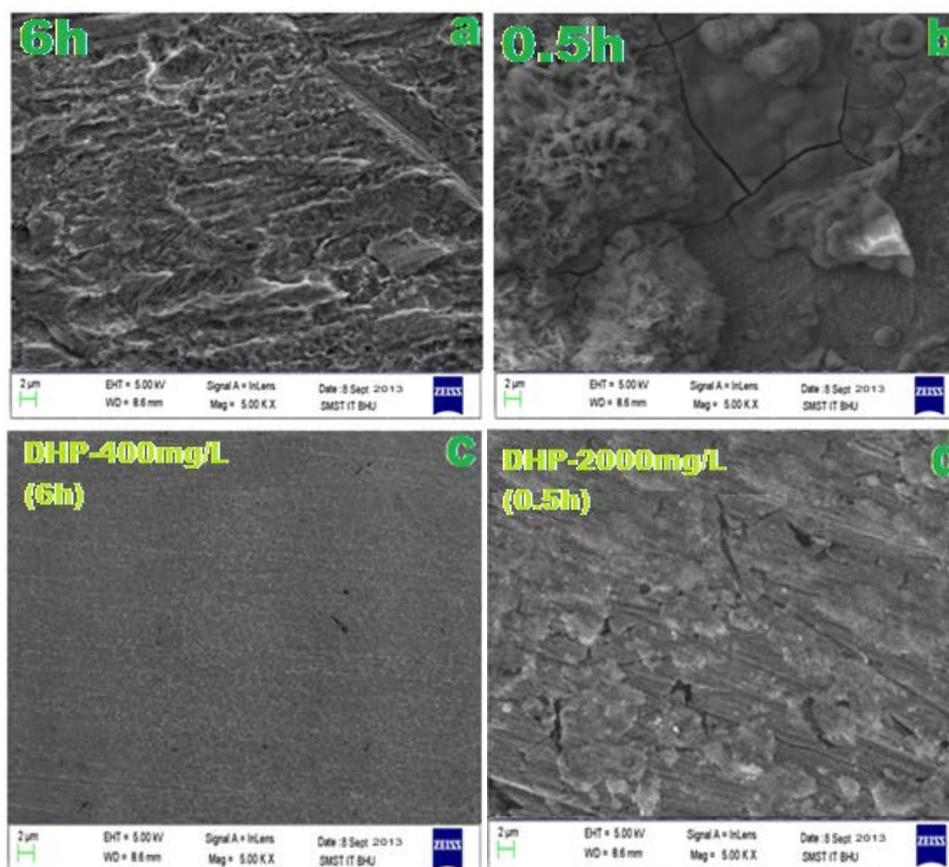
**Fig. 6.** a-d: SEM micrographs of MS surfaces (a) uninhibited 15% HCl (6h) at 308 K (b) uninhibited 15% HCl (0.5h) at 378 K (c) DHP (400 mg/L) for 6h at 308 K (d) DHP (2000 mg/L) for 0.5h at 378 K
