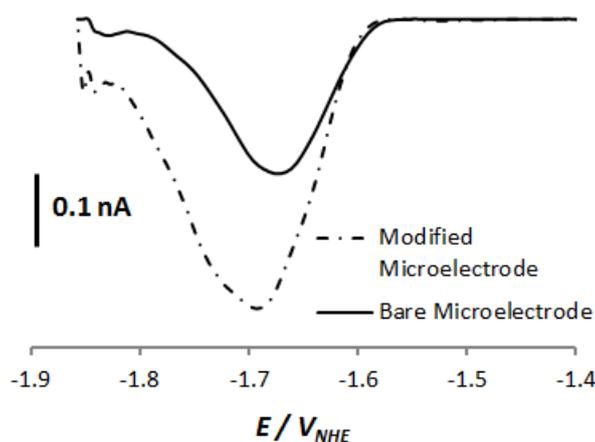
**Fig. 5.** DPV assays of 0.1 mM acetaminophen using bare and mercury thin film modified carbon microelectrode
