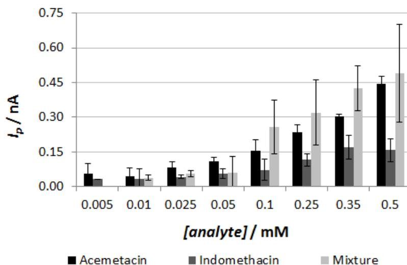
**Fig. 4.** Mean current intensity values of the reduction peaks of (A) acemetacin, (B) indomethacin and (C) its equimolar mixture, attained by AdSDPV. Note: due to background noise during the measurements, it was not possible to obtain the peak current for 0.005 mM of the equimolar mixture
