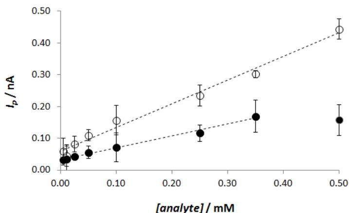
**Fig. 3.** Current intensity values as function of the analyte concentration, for acemetacin (○) and indomethacin (●) attained by AdSDPV
