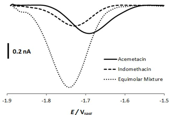
**Fig. 2.** DPV assays of 0.35 mM acemetacin, indomethacin and its equimolar mixture using the modified mercury thin film carbon microelectrode
