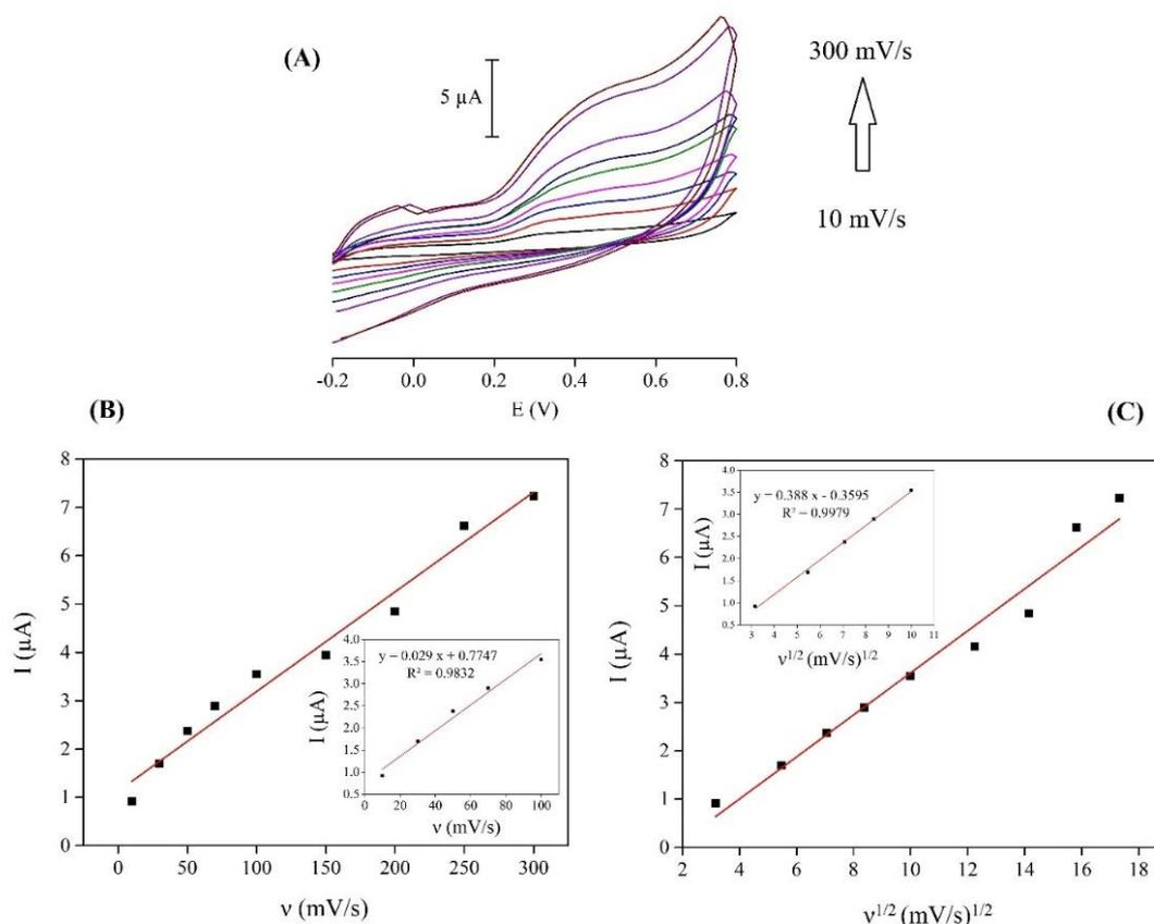
**Fig. 3.** cyclic voltammetry responses of BR ( $40 \mu\text{M}$ ) obtained using CPE at various potential scan rates including: 10, 30, 50, 70, 100, 150, 200, 250 and  $300 \text{ mVs}^{-1}$ (A); the plot of peak current vs.  $v$  (B) and peak current versus  $v^{1/2}$  (C)
