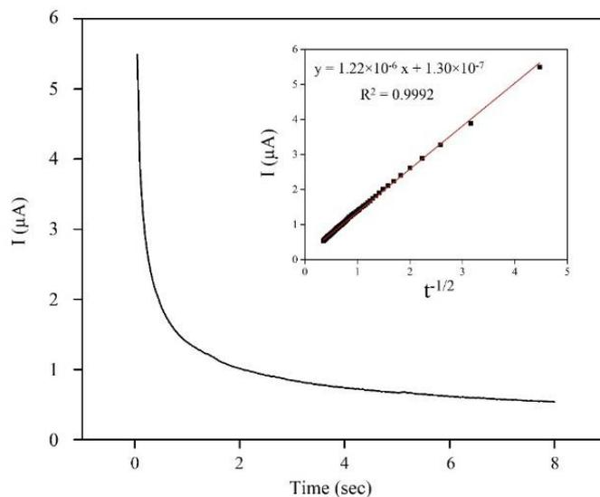
**Fig. 2.** Chronoamperogram of bilirubin (40  $\mu\text{M}$ ) in phosphate buffer (0.05 M, pH 8) at the  $E=0.3$  V; (inset is showing the current signals vs.  $t^{-1/2}$ )
