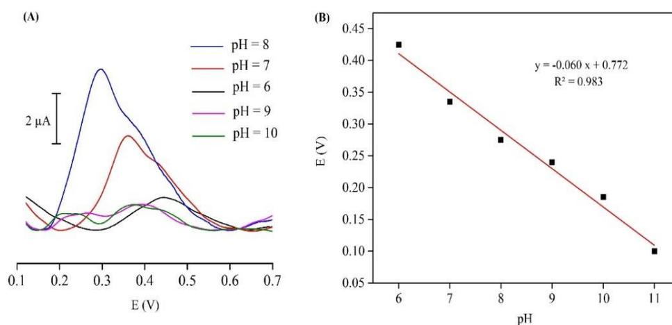
**Fig. 4.** Differential pulse voltammetry signals of the CPE for 20 μM of BR in different pHs (A) and linear relationship of pH vs. peak potential (B); (DPV parameters: pulse time=10 ms, amplitude=100 mV,  $E_{step}=5$  mV)
