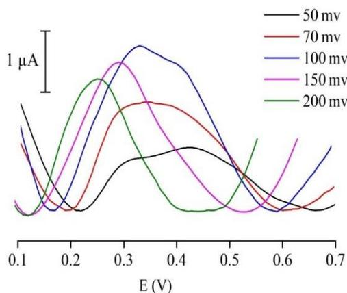
**Fig. 5.** Comparison of DPV responses of CPE in BR (10 μM) for different pulse amplitudes; (DPV parameters: pulse time=10 ms,  $E_{step}=5$  mV)
