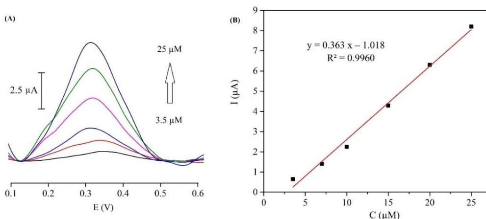
**Fig. 6.** Differential pulse voltammograms obtained from different concentrations of BR using CPE (A) and calibration curve (B) in PBS pH=8 at optimum conditions; pulse time=10 ms, amplitude=150 mV,  $E_{\text{step}}=5$  mV
