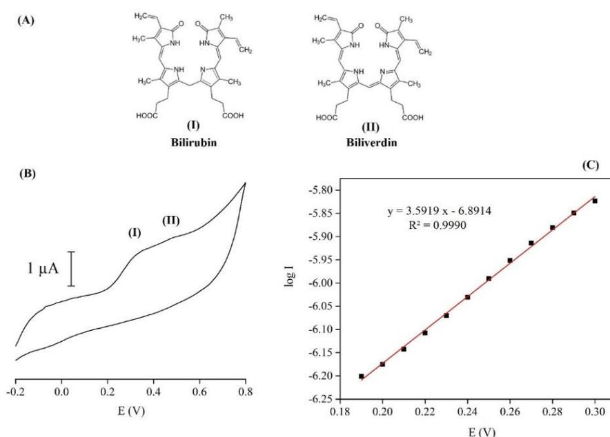
**Fig. 1.** Chemical structure of bilirubin and biliverdin (A), representative cyclic voltammogram of the bilirubin oxidation process in two steps (B) and corresponding Tafel plot (C); (analysis condition: PBS 0.05 M, pH 8, CV scan rate=30 mV/s)
