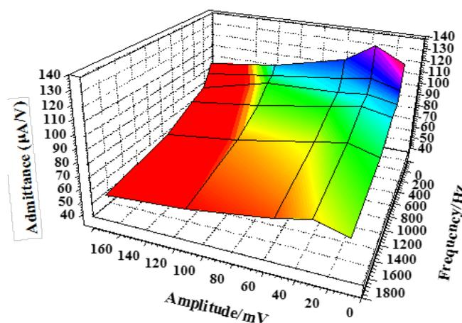
**Fig. 4.** The frequency and amplitude optimization for CPE in NAL 20  $\mu\text{g/mL}$ ; PBS 0.1 M pH=3
