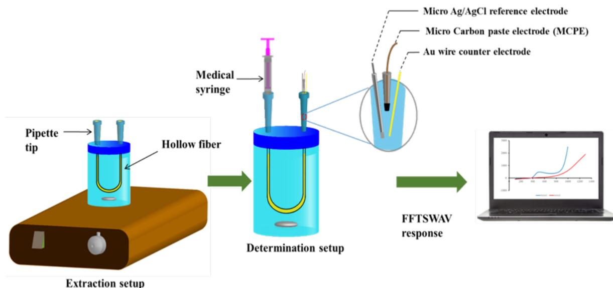
**Fig. 2.** The designed extraction setup for the determination of NAL using EME-FFTASWAV
