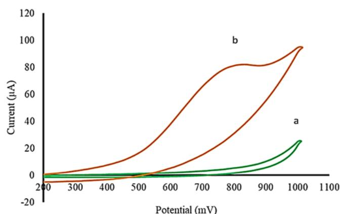
**Fig. 3.** The voltammetric response of the CPE in (a) PBS pH=3, (b) 20  $\mu$ g/mL NAL in 0.1 M PBS pH=3 at scan rate of  $0.5 \text{ V}\cdot\text{s}^{-1}$
