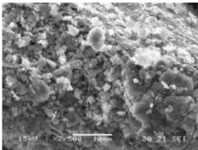
**Fig. 1.** Scanning electron micrograph of Clay paste electrode
