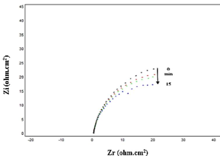
**Fig. 4.** Impedance diagram at different contact times of CPE-Ar with the bacteria
