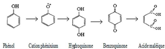
**Scheme 1.** Mechanism of electrochemical oxidation of phenol at Clay-bacteria-CPE
