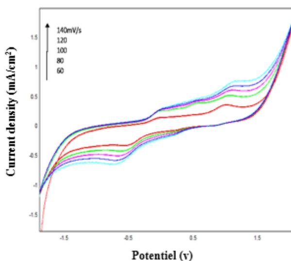
**Fig. 8.** CV's recorded at Clay-bacteria-CPE, in electrolytic medium containing phenol, at various scan rates
