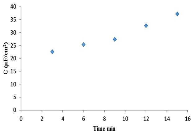
**Fig. 5.** The double layer capacity as a function of the contact time of CPE-Ar with the bacteria
