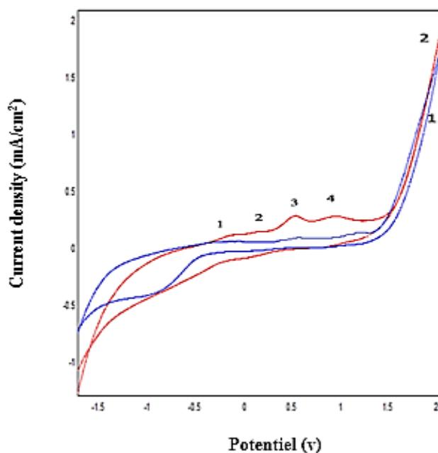
**Fig. 6.** CVs recorded for 4 mM phenol at pH=7 at bare Clay-bacteria-CPE(1) and Clay-bacteria-CPE/phenol (2), scan rate 100 mV/s
