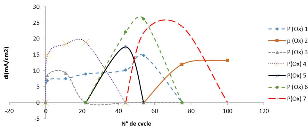
**Fig. 13.** Influence of the current density of the oxidation peaks as a function of the number of cycles recorded by the bacteria-clay-CPE
