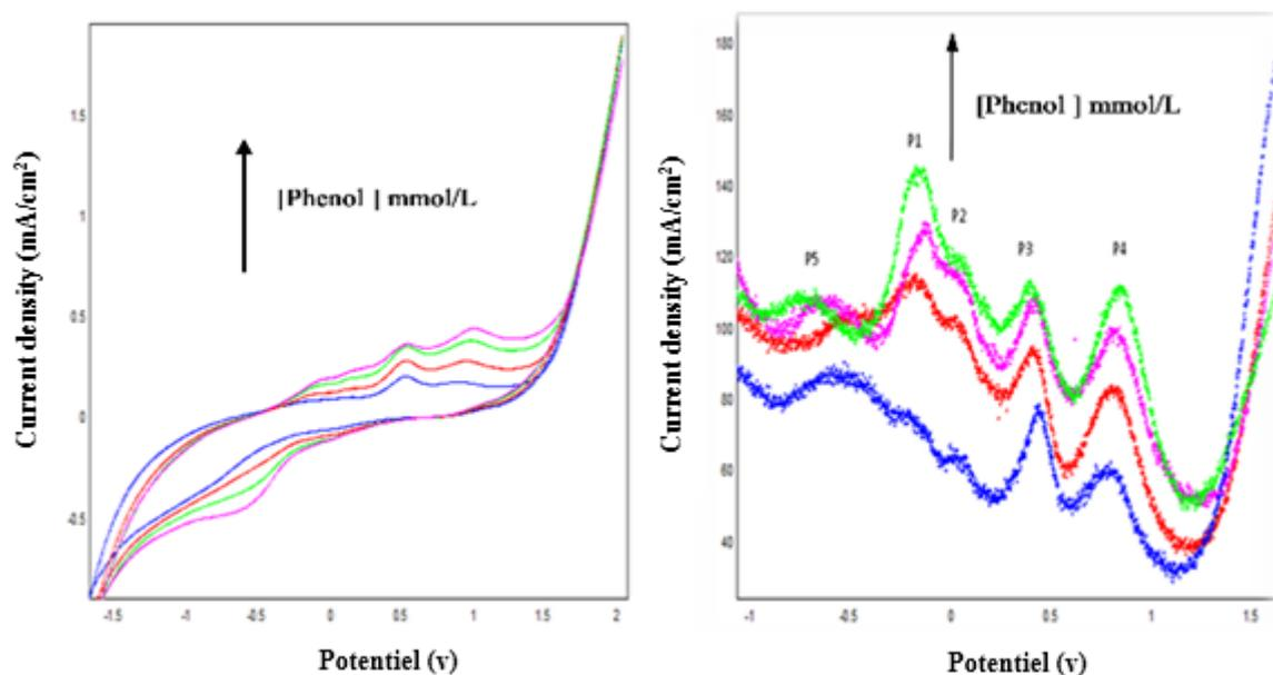
**Fig. 9.** CV's and SQW recorded at Clay-bacteria-CPE, in electrolytic medium containing various concentrations of phenol, at 100 mV/s
