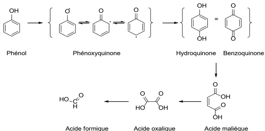
**Scheme 2.** Global mechanism proposed for the electrochemical oxidation of phenol, at bacteria-clay-CPE
