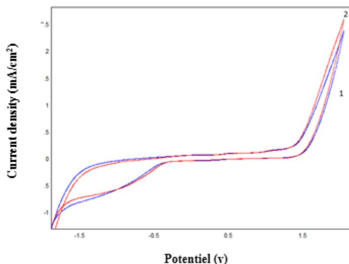
**Fig. 3.** CV's recorded at, 1-Clay-CPE and, 2-Clay-bacteria-CPE, in 0.1 M Na<sub>2</sub>SO<sub>4</sub> solution
