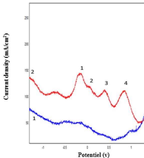
**Fig. 7.** SWV recorded for 4 mM phenol at pH=7 at bare Clay-bacteria-CPE (1) and Clay-bacteria-CPE/phenol (2), scan rate 100 mV/s
