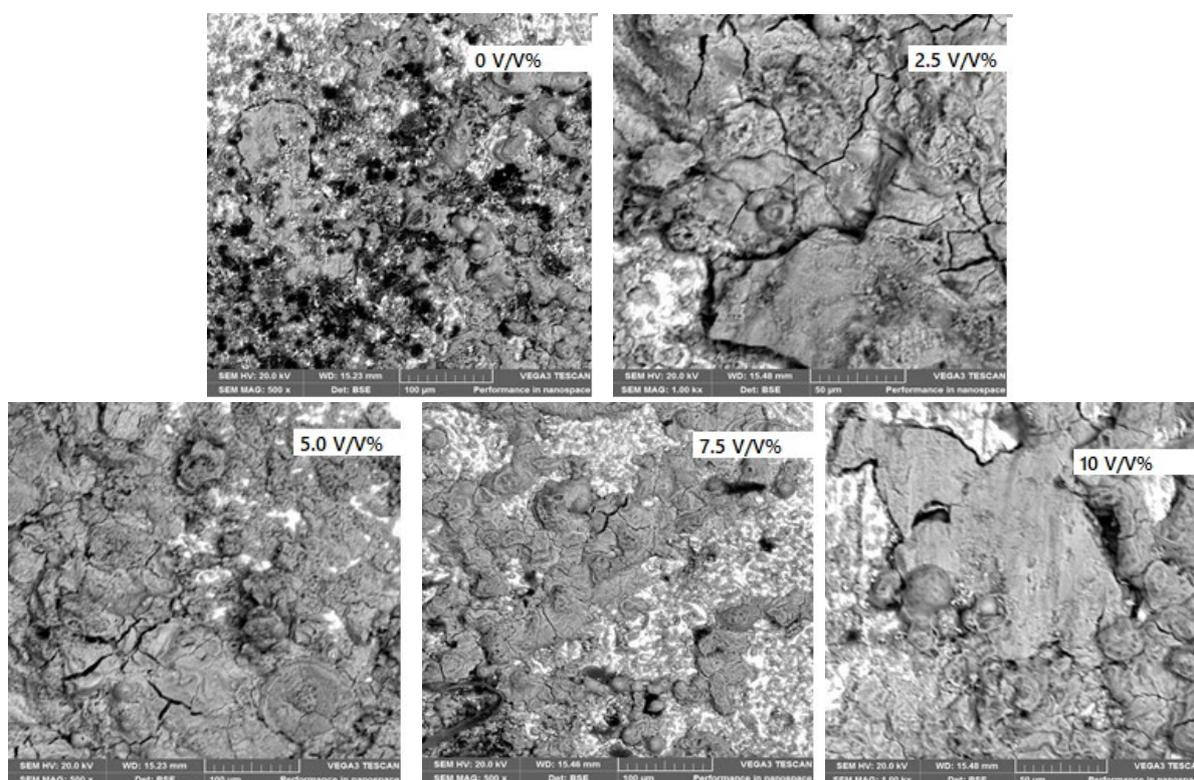
**Fig. 8.** SEM analysis of the surfaces of the mild steel
