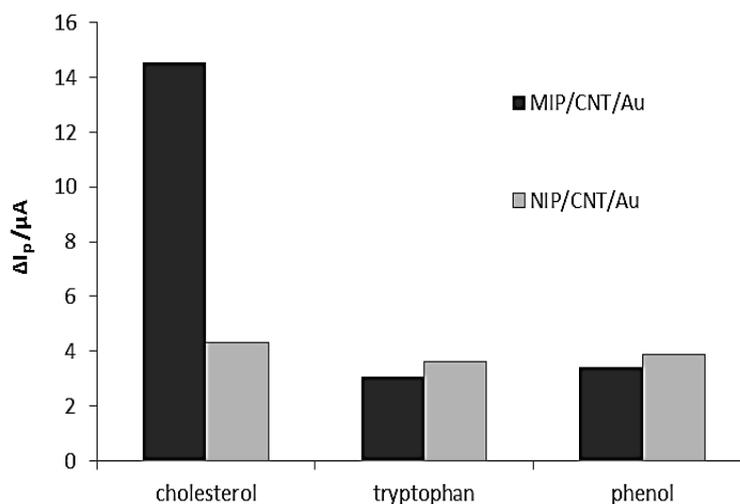
**Fig. 9.** MIP and NIP/MWCNT/Au response to cholesterol ( $100 \text{ mg.dL}^{-1}$ ), tryptophan ( $100 \text{ mg.dL}^{-1}$ ) and phenol ( $100 \text{ mg.dL}^{-1}$ ) in PBS ( $0.1 \text{ M}$ ,  $\text{pH}=7.4$ ).
