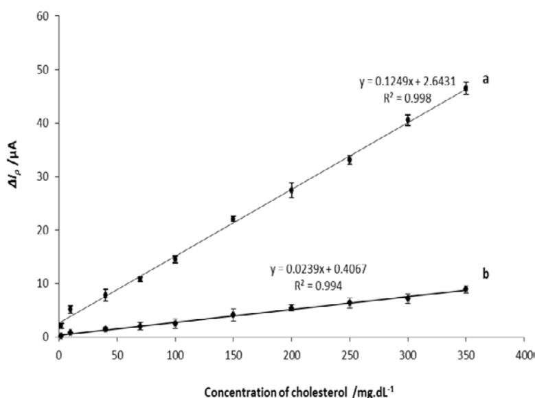
**Fig. 8.** Calibration curves corresponding to the response of the MIP (a) and NIP (b) sensors to the concentration of cholesterol (each point was repeated 3 times)
