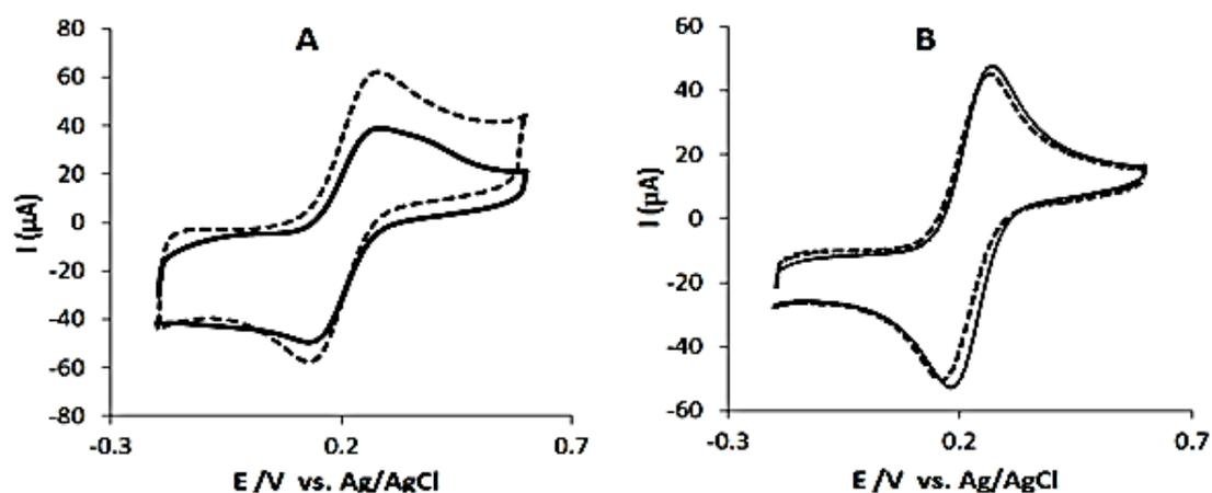
**Fig. 6.** CV response obtained in 5.0 mM KHCF containing 0.1 M of KCl for MIP (A) and NIP (B) modified electrodes after incubation in  $150 \text{ mg.dL}^{-1}$  cholesterol solution for 20 min (dash line) and after 50 min washing electrode for removal of adsorbed cholesterol (solid line)
