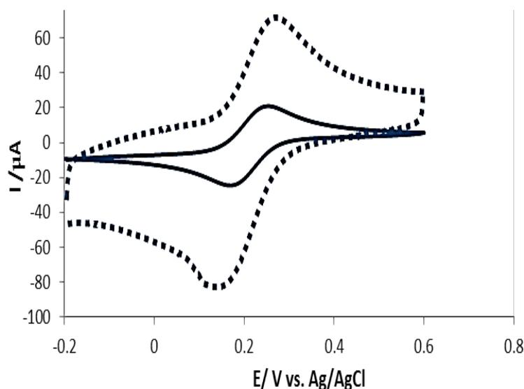
**Fig. 2.** Cyclic voltammograms of Au (solid line) and MWCNT/Au (dash line) in 5 mM KHCF solution containing 0.1 M KCl (scan rate 50 mV.s<sup>-1</sup>)
