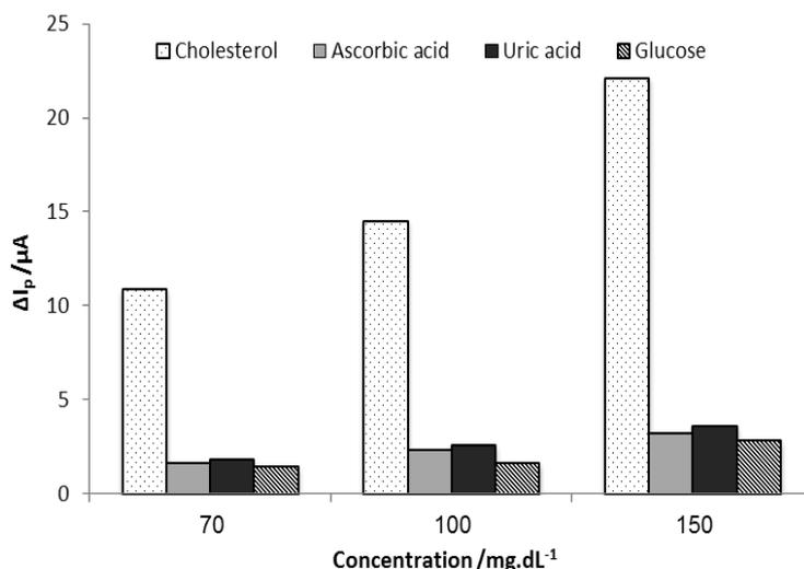
**Fig. 10.** Interference effect of ascorbic acid, glucose and uric acid on the MIP/MWCNT/Au cholesterol sensor
