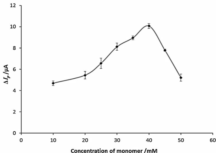
**Fig. 4.** The average  $\Delta I_p$  ( $n = 3$ ) of MIP/MWCNT/Au electrodes in KHCF solution (5.0 mM) containing 0.1 M of KCl. The electrodes are prepared at various concentration of 2-MBI monomer (10, 20, 25, 30, 35, 40, 45 and 50 mM).
