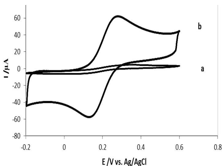
**Fig. 7.** CVs of KHCF (scan rate= $50 \text{ mV.s}^{-1}$ ) on the MIP/Au (a) and MIP/MWCNT/Au (b) electrodes
