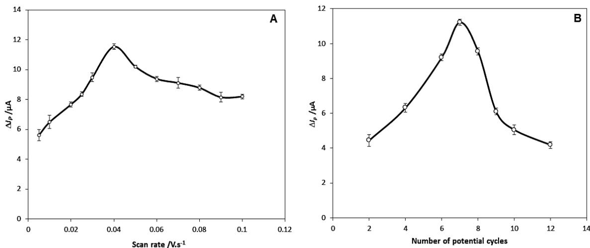
**Fig. 5.** The average  $\Delta I_p$  (n=3) of MIP/MWCNT/Au electrodes in KHCF solution (5.0 mM) containing 0.1 M of KCl before and after removal of cholesterol. The effect of scan rate (5, 10, 20, 25, 30, 40, 50, 60, 70, 80, 90 and 100  $mV.s^{-1}$ ) (A), and the number of potential cycles (2,4, 6, 7, 8, 9, 10 and 12) (B) on the electropolymerization of MIP.
