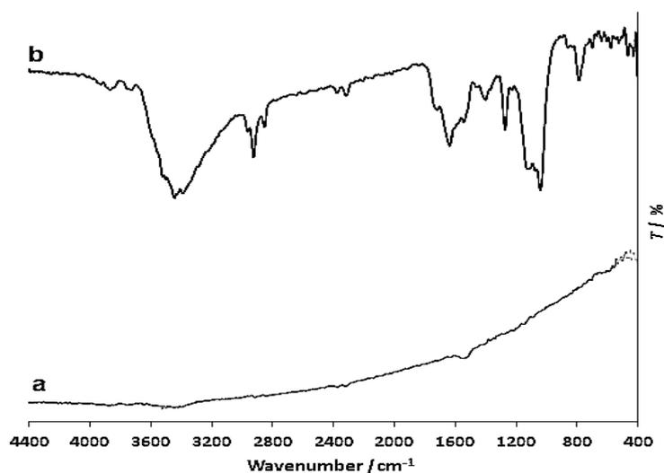
**Fig. 1.** FT-IR spectra of MWCNT (a), and functionalized MWCNT (b)
