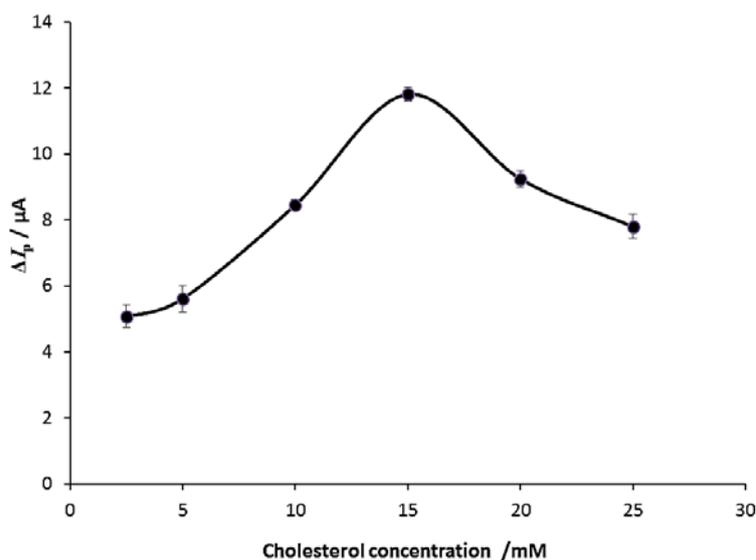
**Fig. 3.** Effect of cholesterol concentration (2.5, 5, 10, 15, 20 and 25 mM) on the MIP/MWCNT/Au electrode response in KHCF solution (5.0 mM) containing 0.1 M of KCl. (Each point was repeated 3 times)
