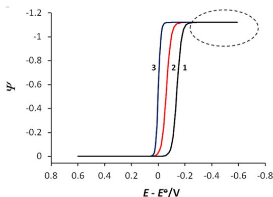
**Fig. 2.** Effect of the kinetics of the electrode reaction ( $\lambda$ ) on the features of cyclic voltammograms, calculated for  $\gamma=1.256$ , and  $\lambda=0.000032$  (1); 0.032 (2) and 32 (3). All the other simulation parameters were the same as those in figure 1
