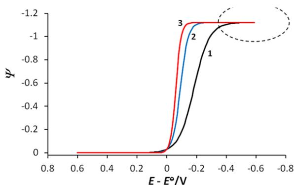
**Fig. 3.** Effect of the number of exchanged electrons in electrode reaction on the features of the cyclic voltammograms calculated for  $\gamma=1.256$ ,  $\lambda=0.032$ , and  $ne=1$  (1); 2 (2) and 3 (3). All the other simulation parameters were the same as those in figure 1
