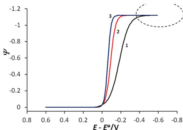
**Fig. 4.** Effect of the electron transfer coefficient of the electrode reaction on the features of the cyclic voltammograms calculated for  $\gamma=1.256$ ,  $\lambda=0.032$ , and  $\alpha=0.25$  (1); 0.5 (2) and 0.75 (3). All the other simulation parameters were the same as those in figure 1
