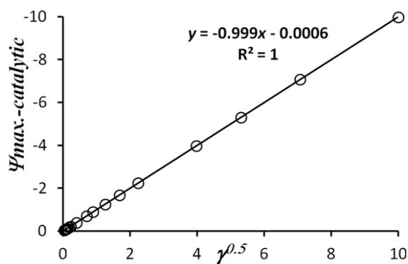
**Fig. 5.** Dependence of the maximal “plateau” catalytic currents of simulated cyclic voltammograms on the square root of the dimensionless catalytic parameter  $\gamma$ . All the other simulation parameters were the same as those in figure 1
