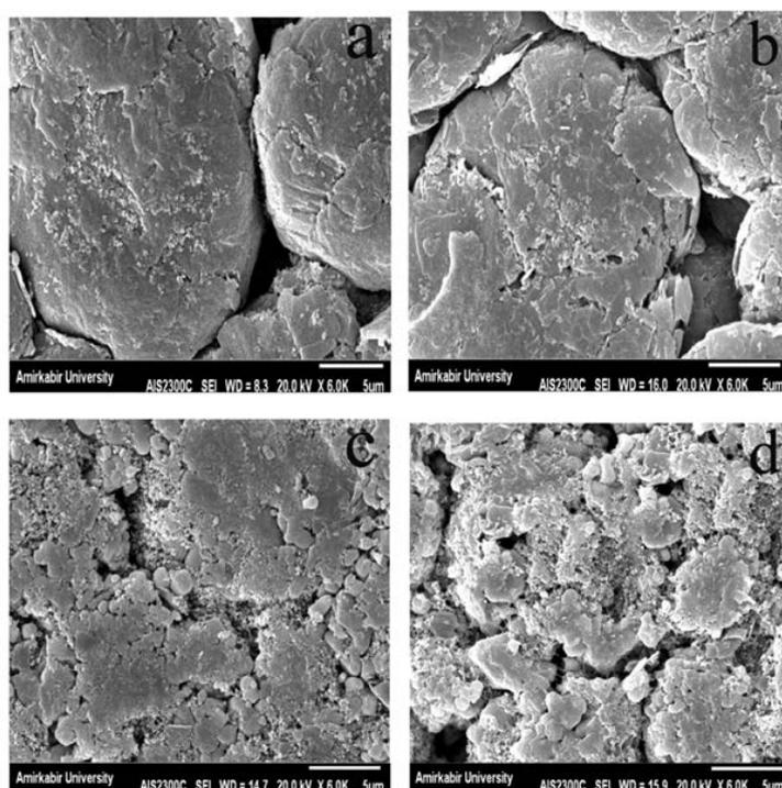
**Fig. 6.** SEM images of Graphite (a) and NMC (c) electrode cycled with electrolyte containing 5% of DMMP and Graphite (b) and NMC (d) electrode cycled with Blank electrolyte
