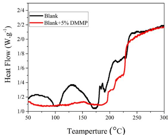
**Fig. 2.** DSC profiles of the two electrolytes: Blank electrolyte (Black Line) and Blank electrolyte +5% vol of DMMP (Red Line)
