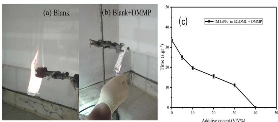
**Fig. 1.** The view of flammability test for electrolyte with DMMP (a); without DMMP (b) and results of SET tests of the electrolytes containing different concentration of DMMP with error bar (c)
