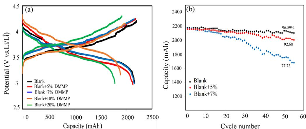
**Fig. 4.** Initial Charge/discharge curves of the cell with blank electrolyte and electrolyte containing different amount of DMMP additive (a) and cycling performance of 18650 cells with Blank electrolyte, Blank electrolyte+5% and Blank electrolyte+7% content of DMMP additive
