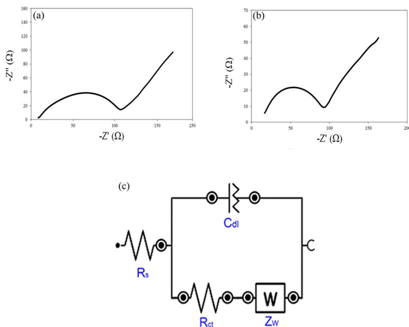
**Fig. 5.** Nyquist plot of half-cell with (a) Blank electrolyte; (b) Blank electrolyte +5 vol.% of DMMP additive and (c) equivalent circuit
