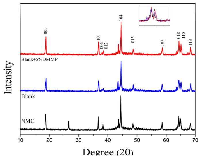
**Fig. 8.** XRD patterns of NMC electrode: prior to the test (Black Line), after cycling with Blank electrolyte (Blue Line) and cycling with Blank electrolyte +5 vol.% DMMP additive (Red Line)
