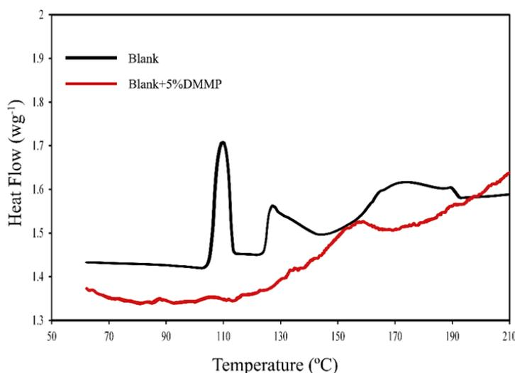
**Fig. 7.** DSC curves of the NMC electrode after cycling with the Blank electrolyte (Black Line) and Blank electrolyte+5 vol.% DMMP additive (Red Line)
