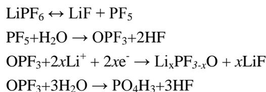
Scheme 1 The auto-catalytic thermal decomposition of LiPF<sub>6</sub>-based carbonate electrolytes [6,7].
