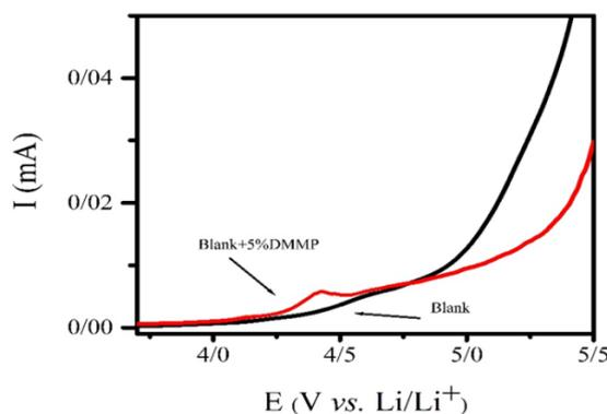
**Fig. 3.** Linear sweep voltammograms of 1 M LiPF<sub>6</sub> EC/DMC (1/1, v/v) solutions without and with 5 vol.% of additives. Pt as the working electrode and Li as the reference and counter electrode. Scan rate is 10 mV s<sup>-1</sup>
