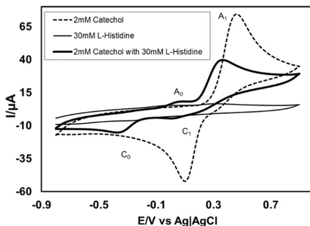
**Fig. 1.** Cyclic voltammogram of 2 mM catechol, 30 mM L-Histidine and 2 mM catechol with 30 mM L-Histidine of Gc electrode in buffer solution (pH 7) at scan rate 0.1 V/s (2nd cycle).  $A_0$  and  $A_1$  is appeared anodic peak and anodic peak,  $C_0$  and  $C_1$  is corresponding appeared cathodic peak and cathodic peak.
