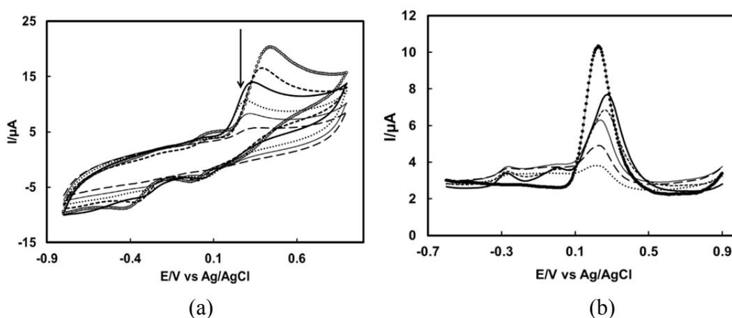
**Fig. 7.** (a) Cyclic voltammogram; (b) Differential pulse voltammogram of 1 mM Catechol in presence of 15 mM L-Histidine of Gc electrode during controlled potential coulometry at 0.4 V in pH 7 at scan rate 0.1 V/s
