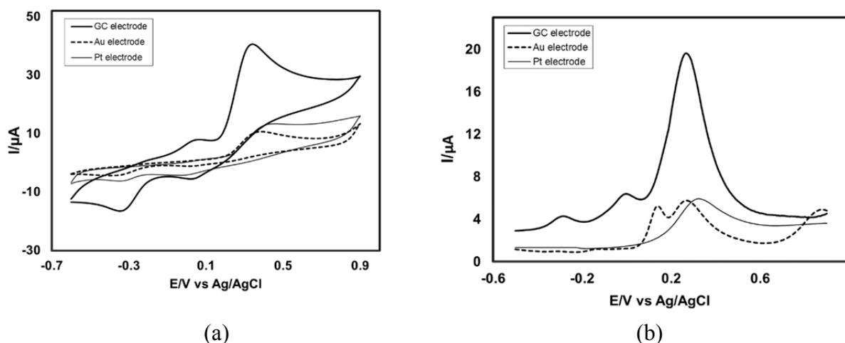
**Fig. 5.** a) CV b) DPV of 2 mM catechol with 30 mM L-Histidine in Gc electrode (3.0 mm), Gold electrode (1.6 mm) and Platinum electrode (1.6 mm) at pH 7 and scan rate 0.1 V/s
