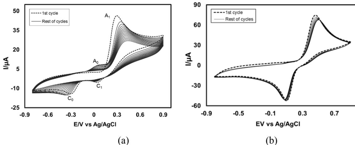
**Fig. 6.** a) CV of 30 mM L-Histidine with 2 mM catechol of Gc (3 mm) electrode in the buffer solution of pH 7 at scan rate 0.1 V/s (15 cycles). The appeared anodic peak current ( $A_0$ ) increased with the iteration scan from the first cycle; b) CV of 2 mM Catechol in the buffer solution of pH 7 at scan rate 0.1 Vs<sup>-1</sup> (15 cycles)
