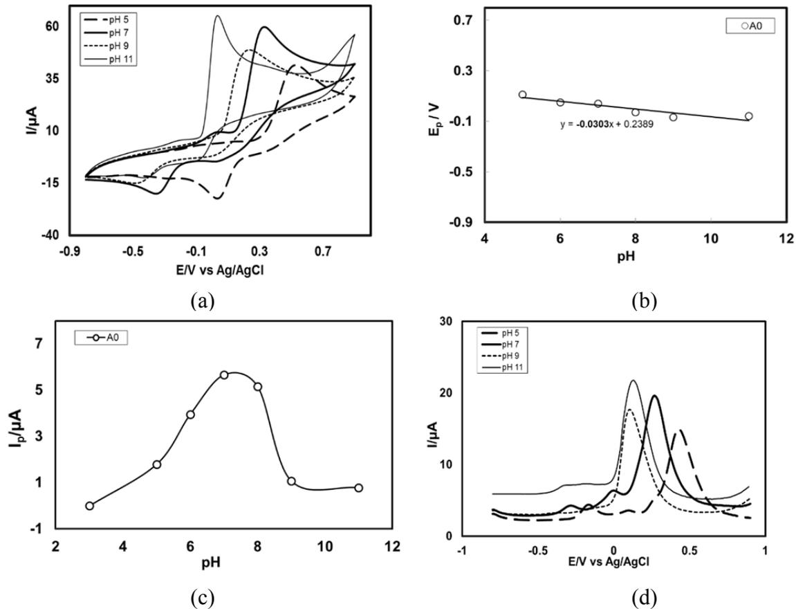
**Fig. 3.** a) CV of 2 mM catechol with 30 mM L-Histidine of Gc (3 mm) electrode in different pH (5, 7, 9, and 11) at scan rate 0.1 V/s; b) Plots of peak potential vs. pH in the same condition; c) Plots of peak current vs pH in the same condition; d) DPV of 2 mM catechol with 30 mM L-Histidine of Gc electrode in second scan of different pH (5, 7, 9 and 11) and scan rate 0.1 V/s. The meaning of symbol  $A_0$  is similar to Fig. 1
