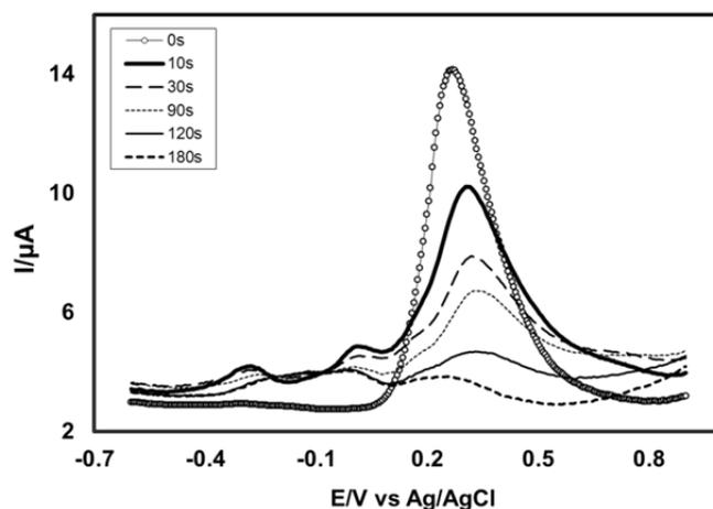
**Fig. 8.** DPV of deposition time change (0, 10, 30, 90, 120 and 180 s) of 2 mM catechol with 30 mM L-Histidine of pH 7 at  $E_{\text{puls}}$  0.02 V,  $t_{\text{puls}}$  20 ms and scan rate  $0.1 \text{ Vs}^{-1}$
